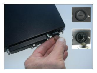
3. If you are replacing the old battery, remove it from the battery compartment.
