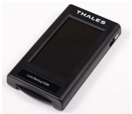
The Luna Backup HSM 7 is available in the following models. All models can be initialized in multifactor quorum or password-authenticated mode for backing up either multifactor quorum or password authenticated partitions. In-field storage upgrades are not available.
