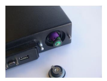
**5.** Use the battery compartment cover to push the battery into the compartment, aligning the tabs on the cover with the compartment slots. Twist the cover clockwise to lock the compartment.
